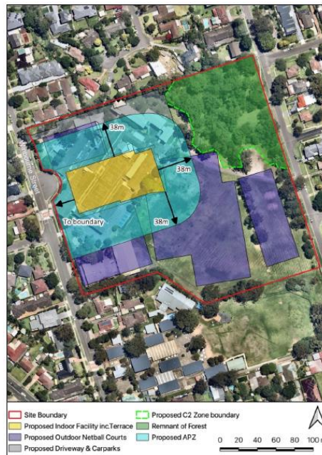
Figure 17: Proposed Asset Protection Zone (APZ) map recommending the building (yellow) is protected by a 38m inner protection area (IPA) (blue).
