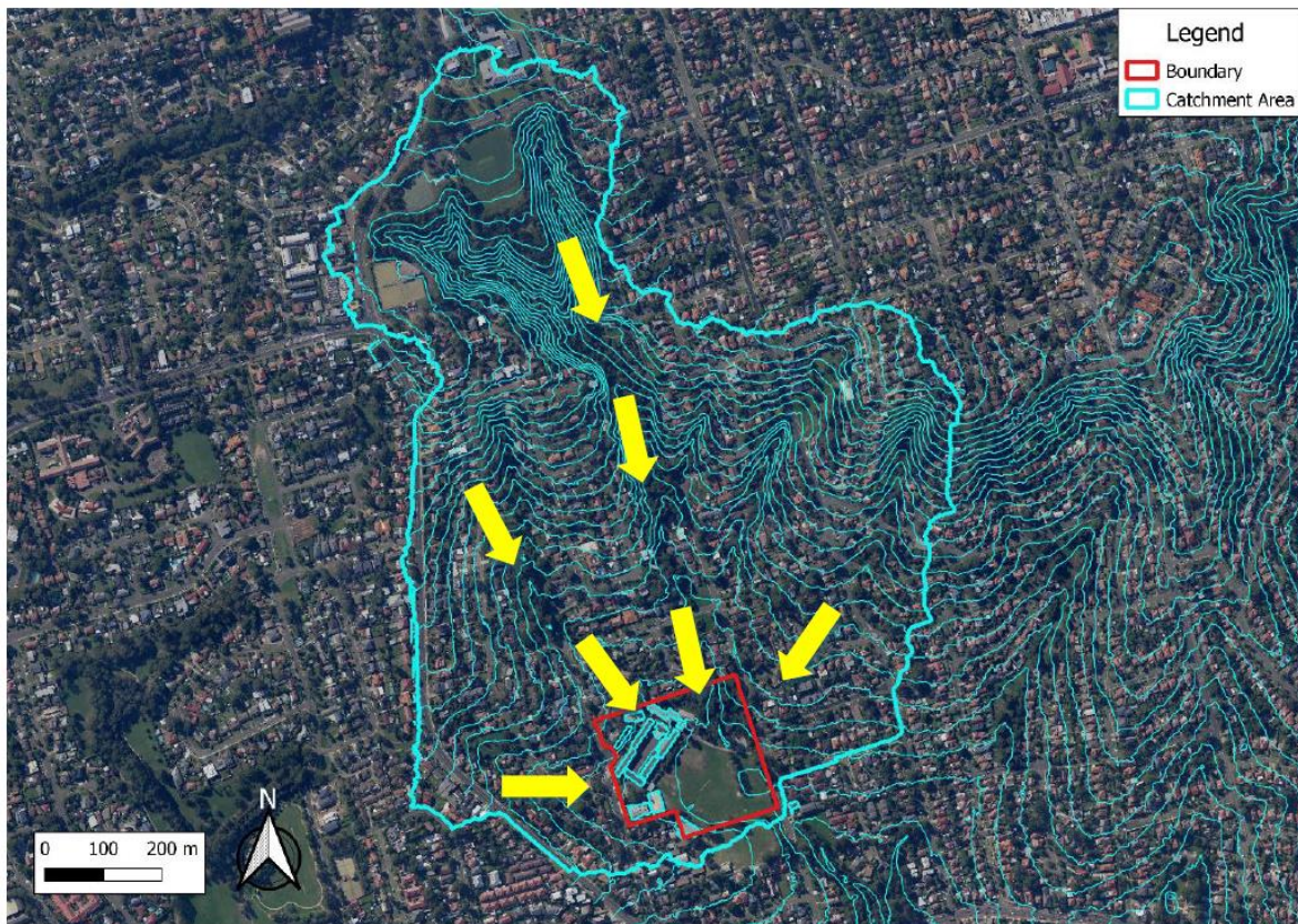
Figure 7: Extract from the Flood Impact Statement prepared by Quantum Engineers showing the overland flow ‘Contributing’ Catchment Plan from the localised upstream catchment.
