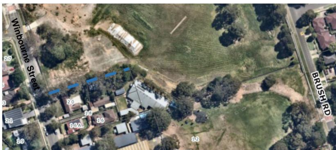
Figure 29: Aerial view of the site showing the location of the 2m high acoustic barrier (blue) along part of the southern boundary shared with residential properties and part of Ermington Public School.
