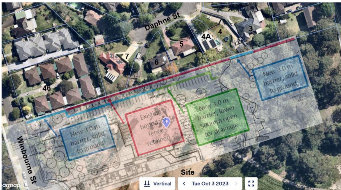
Figure 41: Overlay of the acoustic barrier scheme proposed by the Applicant's acoustic consultant over an aerial view of the site. This overlay indicates where the existing boundary fence is proposed to be retained (red), where a new 3m high acoustic barrier is proposed on the boundary and set back behind buffer landscaping (blue and green).
