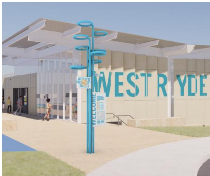
Figure 13: Example of a proposed Entry Totem ID sign a total height of 4.5m including the feature 'hoops.' The signage specifies the direction of groups of courts and a site directory. Business identification signage 'West Ryde' is shown on the façade fronting Winbourne Street.
